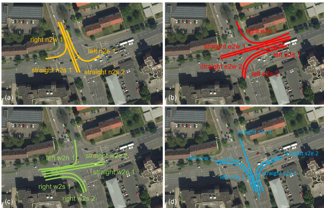
Figure 3. Urban intersection with 19 different traffic manoeuvres: The subfigures show routes by direction: (a) orange from north, (b) red from east, (c) green from west, (d) blue from south.
