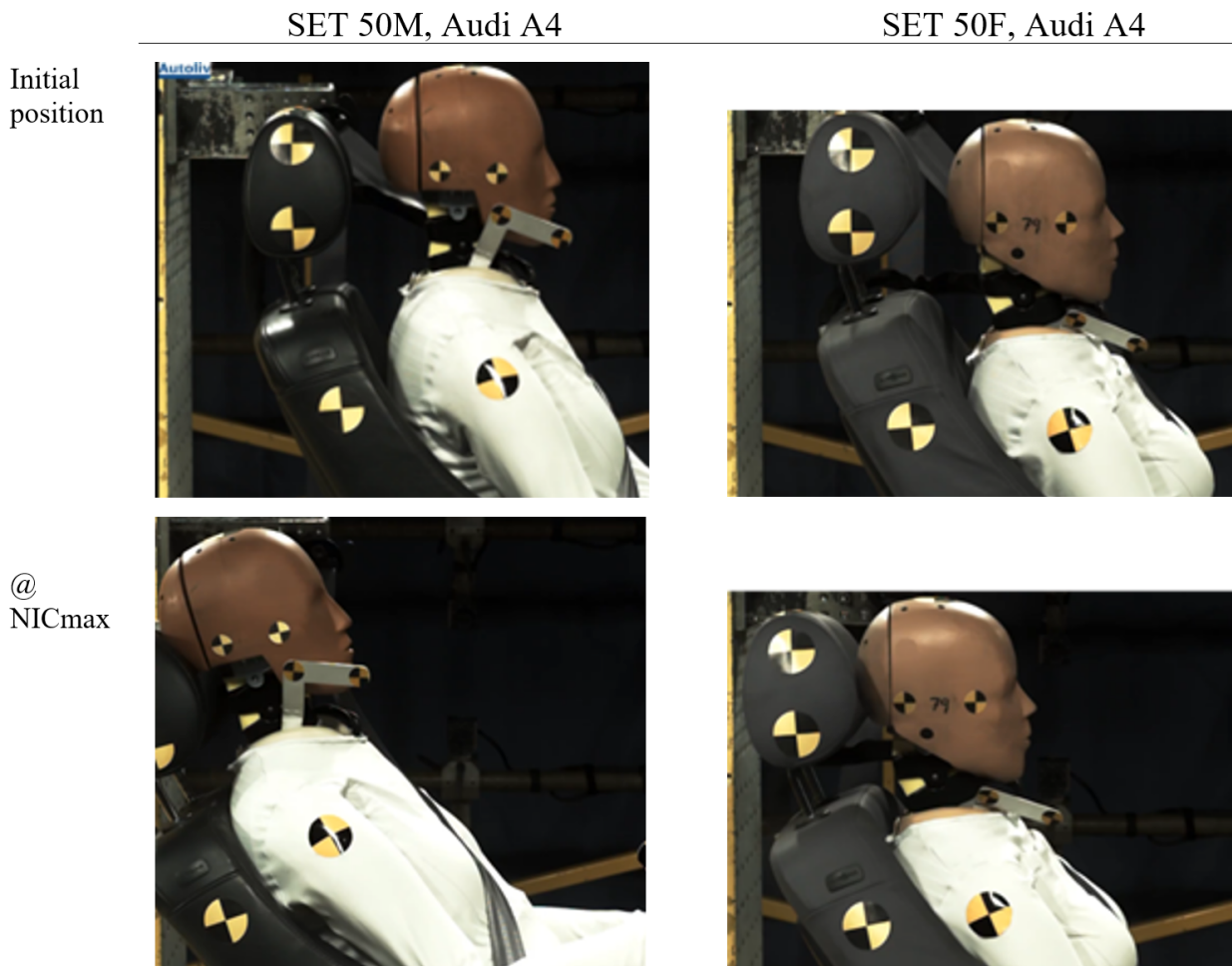
Figure 5. SET 50M (left) (top) and SET 50F (right) in the Audi A4 seats, initial position (top) and at the occurrence of NICmax (bottom) from the high-speed video of the impacts. Picture credits: Autoliv.
