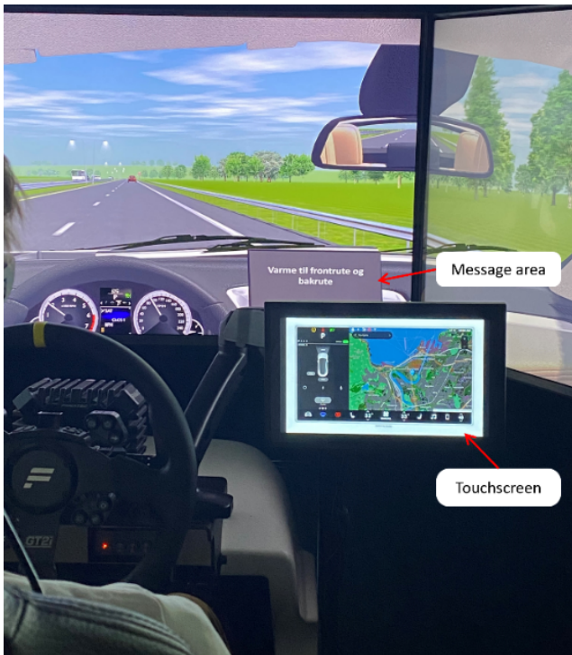
Figure 1. Fixed-base driving simulator with an in-vehicle touchscreen.
