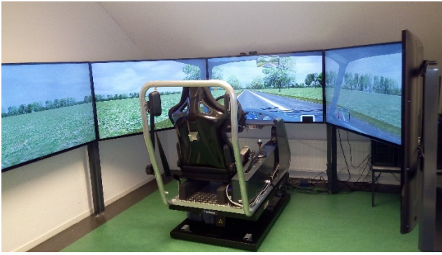
Figure 1. The driving simulator with moving base
