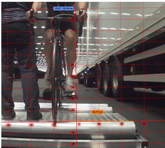
Figure 6. A screenshot illustrating the position tracking; the current position of the edge of the front wheel is 16.78 cm to the left of the targeted mean position (at “0”).
