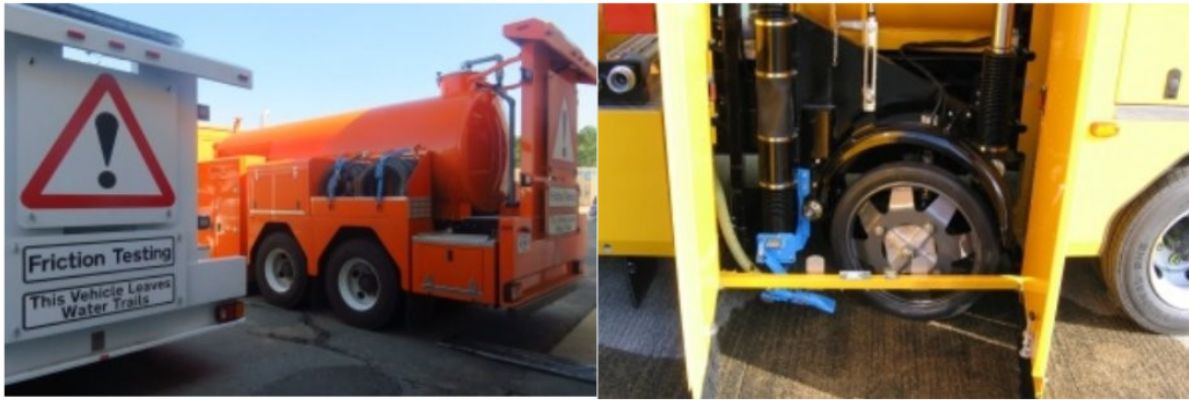
Figure 3 SCRIM machine used for collecting pavement friction data and supplementary information
