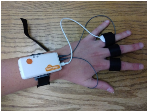
Figure 1 Shimmer3 GSR+ sensors (shown attached to three fingers) send data to a host computer through the wireless transmitter (shown attached to the wrist) in real time.
