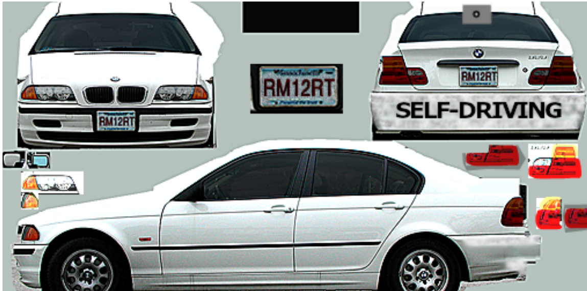
Figure 3 Screenshot of the RGBA image file edited using GIMP to modify pre-loaded dynamic vehicles from SimCreator
