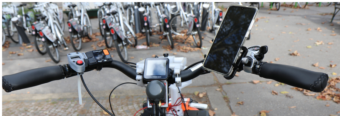
Figure 4 Sensor setup for acceleration data collection. The Xiaomi Mi 9X smartphone can be seen attached to the right half of the handlebar. The round dark grey device on the handlebar stem is the XSens MTI-680G, containing an industrial grade IMU and GNSS sensor. As can be seen, the XSens is slightly tilted upwards, yielding an IMU z-axis slightly pointing backwards towards the rider. The Smartphone on the other hand is tilted back and to the left, resulting in an IMU z-axis pointing approximately towards the riders left shoulder.
